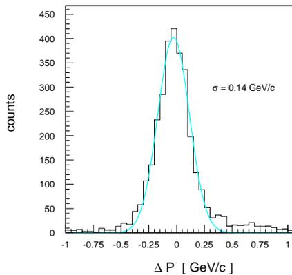
Fig. 1: Difference between generated ( $P_{gen}$ ) and reconstructed ( $P_{rec}$ ) neutron momenta for the  $dp \rightarrow ppn_{sp}$  reaction simulated at a deuteron beam momentum of 3.204 GeV/c. At this beam momentum an average momentum of specatator neutrons is equal to 1.6 GeV/c.
