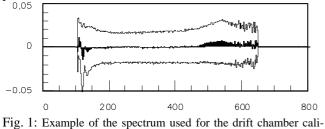
bration. Shaded area presents mean values of  $\Delta X$  (in cm) as a function of the drift time (in ns). Upper and lower histograms indicate a band of one standard deviation of the  $\Delta X$  distribution.
