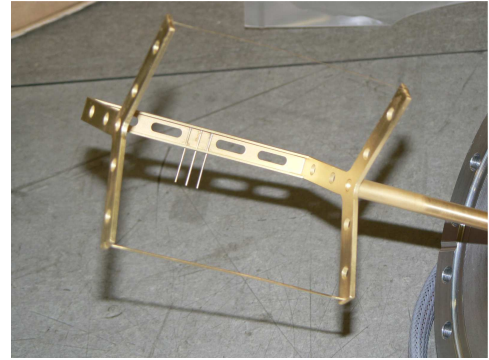
Fig. 3: Photograph of the wire device for precision measurement of the cluster target dimensions. The rotation axis of the device is mounted perpendicular to the cluster jet.
