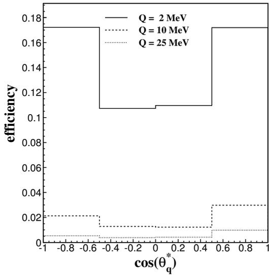
Figure 7: Experimental efficiency for registering and identifying the  $pp \rightarrow pp\eta$  reaction at  $Q = 2$  MeV (solid line),  $Q = 10$  MeV (dashed line), and  $Q = 25$  MeV (dotted) presented as a function of the polar angle of the  $\eta$  meson emission in the centre-of-mass system.
